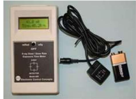
The Model 8900 automatically resets at the beginning of each exposure, holding the reading until the next exposure. There is no need to reset the meter before each measurement.
