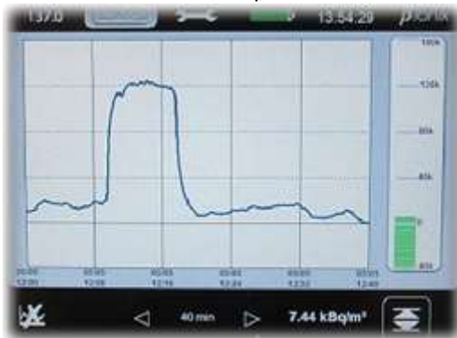
example of the response \beta ionix 3 - MES Volume activity measured 100 kBq/m 3
