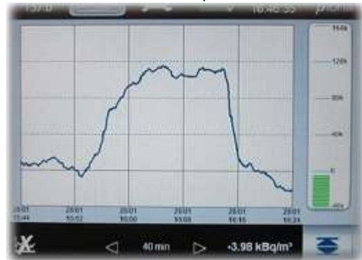
example of the response \beta ionix 3 - CMP Volume activity measured 100 kBq/m 3
