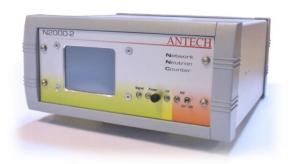
The N2000-2 also provides a High Voltage output, which can be set in a range of 0 - 2000Vdc and is provided through an SHV output bulkhead. The High Voltage output is controlled through a software switch in the system setup and is inhibited by a hardware switch on the front panel. The HV status is indicated by a red LED.
